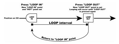
Note: The "LOOP OUT" point will be erased if "LOOP IN" is pressed or a new "CUE" point is set after the "LOOP OUT" point.
